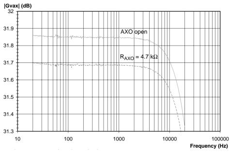
Fig.27 Gain of the auxiliary amplifier
