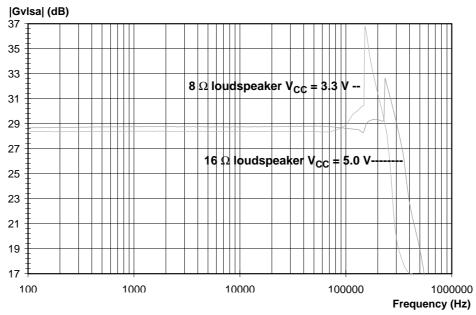
Fig.29 Gain of the loudspeaker amplifier at two output loads
