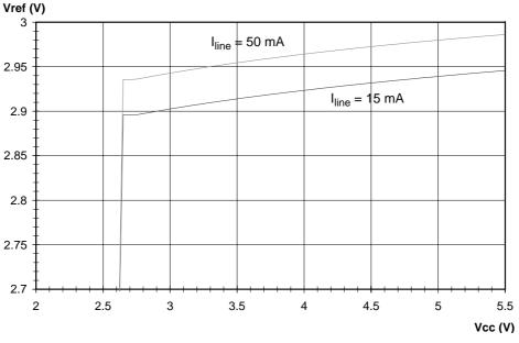
Fig.6 Dependency of  $V_{REF}$  with the supply voltage  $V_{CC}$
