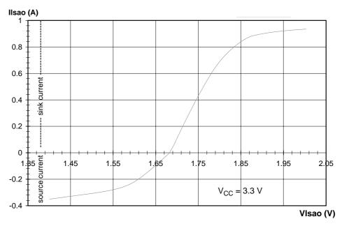
Fig.33 Output current capability at  $V_{CC}$  = 3.3 V
