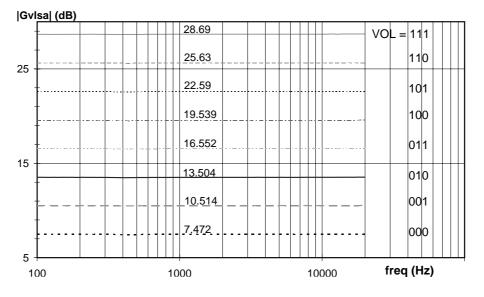
Fig.37 LSA gain versus VOL control setting
