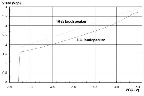
Fig.32 Output voltage capability of the loudspeaker amplifier
