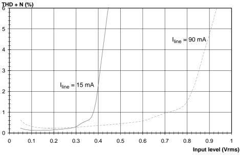
Fig.22 Distortion of the line signal versus input level of TX amplifier
