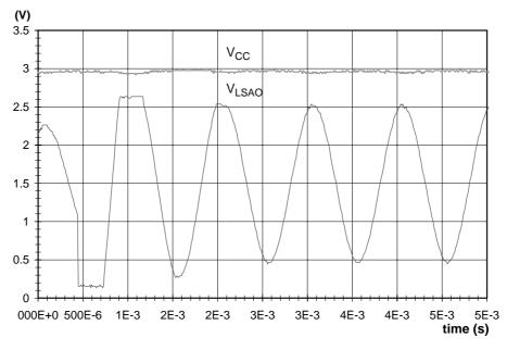
Fig.34 Attack control of the loudspeaker signal at overdrive of the input level
