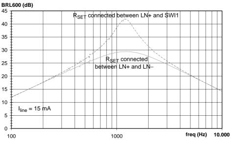
Fig.18 BRL at VRM;  $Z_{\mbox{\scriptsize SET}}$  realised at two ways
