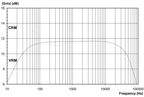
Fig.19 Gain of the transmit amplifier at VRM and CRM
