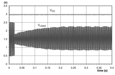
Release of the loudspeaker signal when V<sub>LSAI</sub> is reduced from 63 mVrms to 20 mVrms is shown in Fig.35.
