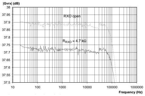
Fig.23 Gain of the receive amplifier
