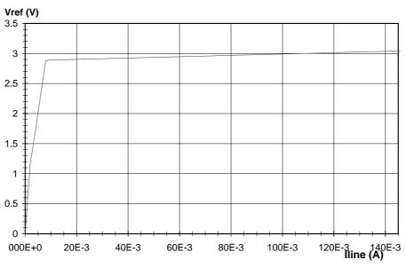
Fig.4 Reference voltage between LN and SLPE versus Iline
