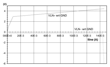
Fig.10 Activated current protection at I<sub>line</sub> > 144 mA
