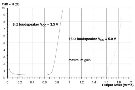
Fig.31 Distortion of the loudspeaker signal caused by the output level at max. gain
