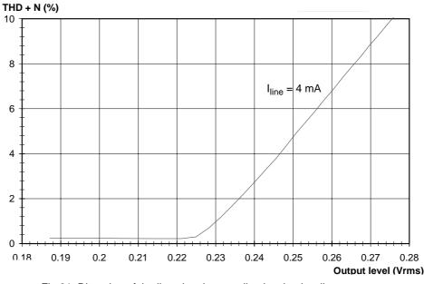
Fig.21 Distortion of the line signal versus line level at low line current
