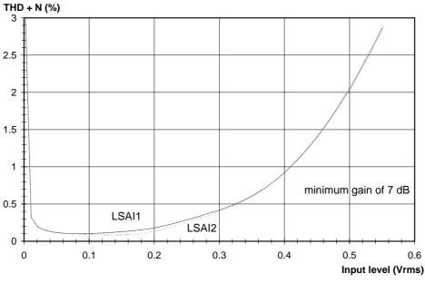
Fig.30 Distortion of the loudspeaker signal caused by the input level at min. LSA gain
